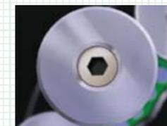
By loosening the retaining bolt the Disc-Blades can be rotated in either direction. If damage occurs to the blade through insertion of contaminants i.e. stones, nails etc, the damaged section can be simply positioned away from the cutting area.
